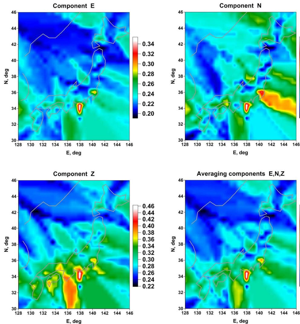
Averaged maps of maximum normalized eigenvalue (divided by the sum of all the eigenvalues) of the correlation matrix for the 3-component GPS measurements in Japan with a time step of 5 minutes are presented.
