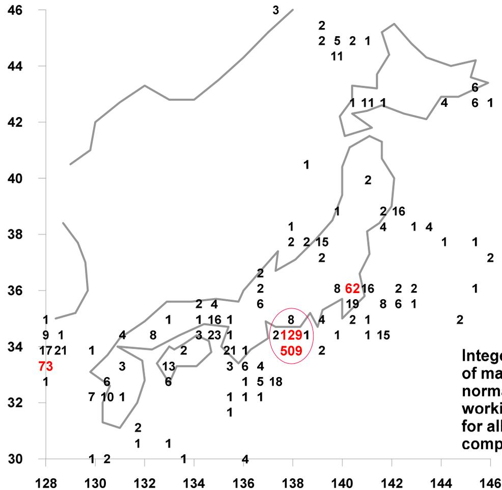
Graphic of sequential maximal values of maximum normalized eigenvalue of correlation matrix within nodes of regular grid 30x30 for each 5 days elementary map and for each GPS component (E, N and Z).
